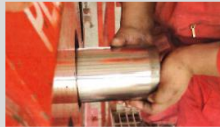
Fig. 3 - Installation of plunger.
