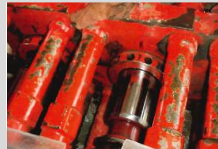
Fig. 4 - Gland nut tightened back to alignment mark.
