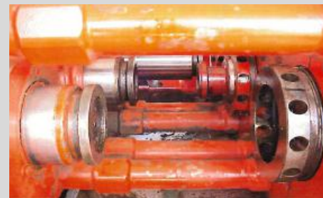
Fig. 2 - Gland nut backed off.
