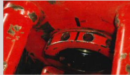
Fig. 1 - Alignment mark with packing hand tight plus 1/4 turn with no plunger.
